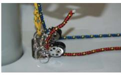
9 Feed the red Vectran control line (part 4) through the port deck turning block.
