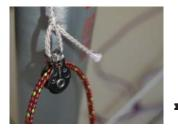
**10** Continue to feed the Vectran control line through the block tied to the mast at the gooseneck.
