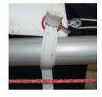
22 The strap is pulled so that the clew of the sail is tight to the boom, but can still slide when adjusted by the outhaul. The velcro is secured down.
