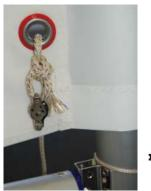
1 Tie the **block and becket** to the **6 mm Vectran x 1.2 m** (part 6) length and feed it through the cunningham eye of the sail from the starboard side.
