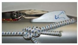
**25** Tie off the bungee around the boom forward of the cleat with a bowline.
