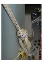
Tie a bowline around the boom vang tang with the vang in place.
