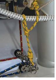
Finally tie the mast retention line (part 5) to the tang and the block plate so that the mast can rotate 180 degrees and the bowline acts as a fairlead for the daggerboard bungee below the vang.
